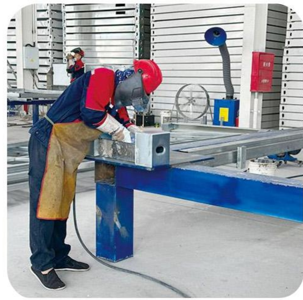
双翼箱角焊接 (Biplane box corner welding)
